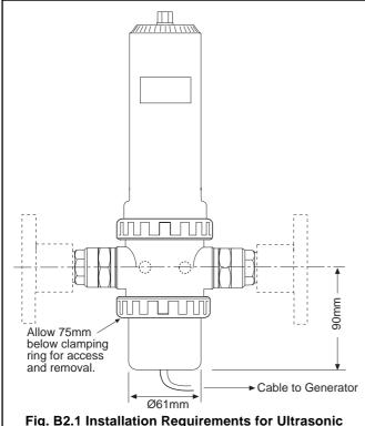
Fig. B2.1 Installation Requirements for Ultrasonic Transducer in 'Flow' Electrode System
