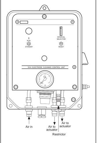
Fig.C3.4 Controls, Indicators and Mechanical Interconnections on Model 7610 Wiper Control Unit
