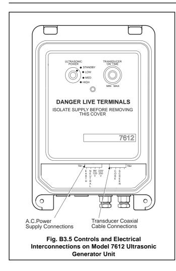
When the electrical connections to the generator unit have been satisfactorily completed, and the modified electrode system reinstalled at its sampling point, the ultrasonic cleaning system can be set in operation by simply turning the front panel control switch from STANDBY to one of the three available power levels - LOW, MEDIUM or HIGH. Refer to Fig. B3.5.
