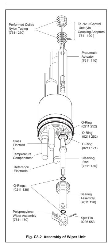
Warning. Always ensure in the case of in-line systems that the sample line pressure is reduced to zero before removing the electrode assembly from the sampling point.
