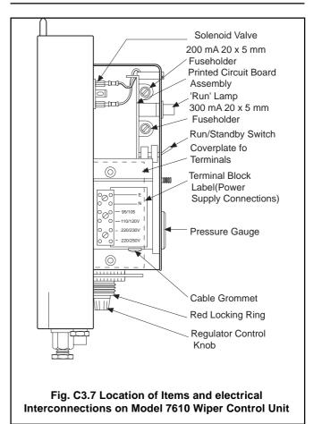
b) Pull the red locking ring downwards to disengage it, and slowly turn the black control knob clockwise until the pressure gauge indicates an operating pressure of 4 bars (58lbfin<sup>-2</sup>) approx. For long pipe runs over 30 metres (98ft) it is recommended to open the pressure regulator fully so that the gauge indicates the inlet pressure supply of 6.9 bars (100 lbfin<sup>-2</sup>).
