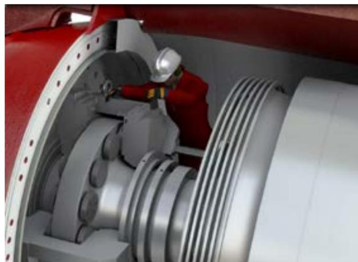
The propeller bearing is of the roller type, but the Azipod unit's shaft thrust bearing is available with both roller and hybrid types depending on the size of the Azipod unit. Hybrid type bearings enable enhanced life cycle cost performance and reliability in icebreaking. Hybrid type thrust bearing pads (to stop wear) can be changed from inside the Azipod unit without dry-docking the ship or pulling out the Azipod module's shaft.
