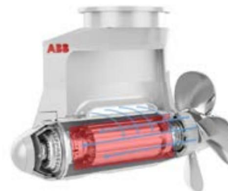
Propeller and thrust bearings are of the roller type. Propeller and thrust bearing are directly cooled by the surrounding water through the steel structure. The propeller bearing is automatically grease-lubricated.
