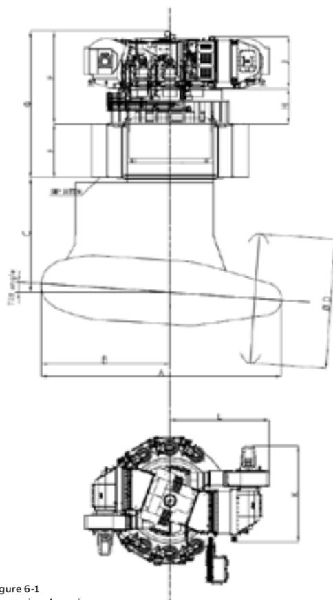
Figure 6-1 Dimensional nominations for the Azipod propulsion system
