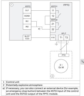
With an FSO module, one-channel connection. This connection is SIL 1 capable (no redundancy between STO channels).
