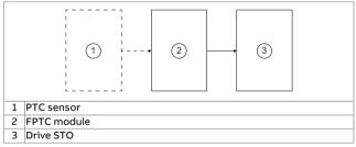
This diagram is applicable to configuration 5. See Wiring example 5 (page 44).
