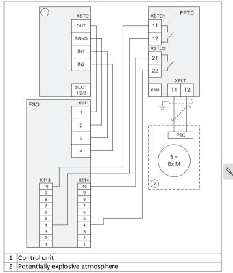
With an external safety relay, two-channel connection. This connection is SIL 2 capable (redundancy between STO channels).
