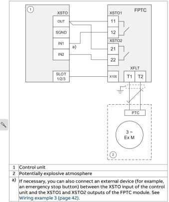
With an FSO module, two-channel connection. This connection is SIL 2 capable (redundancy between STO channels).
