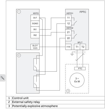
One-channel connection. This connection is SIL 1 capable (no redundancy between STO channels).
