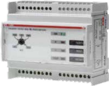
In IT electrical distribution networks with isolated neutral, and in PV networks particularly, the high insulation impedance prevents earth faults from generating currents that would dangerously elevate the potential of exposed conductive parts. Therefore, in case of earth leakage, in an IT network it is not necessary to interrupt the supply, but it is still essential to monitor the insulation level in order to detect faults and restore optimal functioning of the system.
