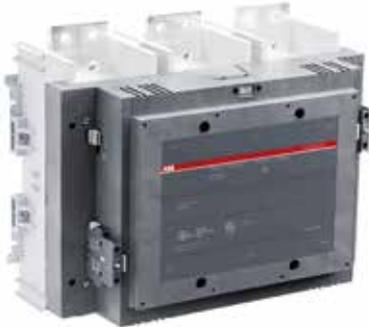
The AF..T range is specially designed for renewable energy AC switching applications with “Low-voltage Ride Through” function. The AF..T contactor is able to withstand a voltage drop on the control voltage without opening. The built-in drop-out delay circuit provides enough energy for the coil voltage to remain above the drop-out level.
