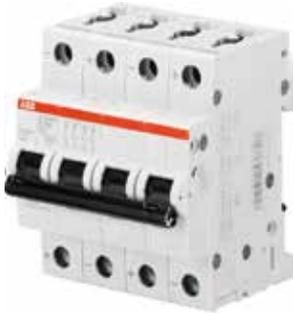
The S200 M UC Z range of miniature circuit-breakers features permanent magnets on the internal arcing chutes able to extinguish an electric arc of up to 440 V DC acc. to IEC 60947-2 with  $I_{cu} = 10$  kA. However, use of these components establishes circuit-breaker polarity, thus they must be powered in a certain direction. A diagram showing how the string and inverter must be connected is given alongside.
