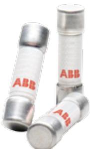
The E 9F PV range of cylindrical fuses has been designed to protect DC circuits up to 1000 V DC according to gPV trip characteristic specific for PV systems. E 9F PV 10.3 x 38 mm fuses offer the best solution for protecting strings, inverters and surge arresters in photovoltaic systems with nominal currents up to 30 A.
