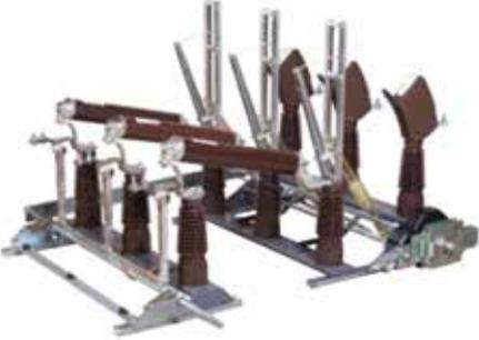
NALFWind is a 36 kV air-insulated switch-fuse combination for protection of distribution transformers in renewable installations. It is equipped with fast-acting ABB CEF-S current limiting fuses that provide protection on both MV and LV sides for transformers up to 3,000 kVA.
