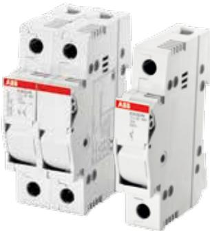
The E 90 PV series of fuse disconnectors has been designed for up to 1000 V DC applications in DC-20B category. The E 90 PV series is specifically focused on overcurrents protection of photovoltaic systems. It provides a reliable, compact and effective solution due to its 10.3 x 38 mm gPV cylindrical fuses.
