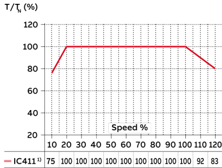
Figure 12. Increased safety synchronous reluctance motors Ex ec T3, cast iron dust ignition protection synchronous reluctance motors Ex t T125°C; nominal frequency of motor 50Hz
