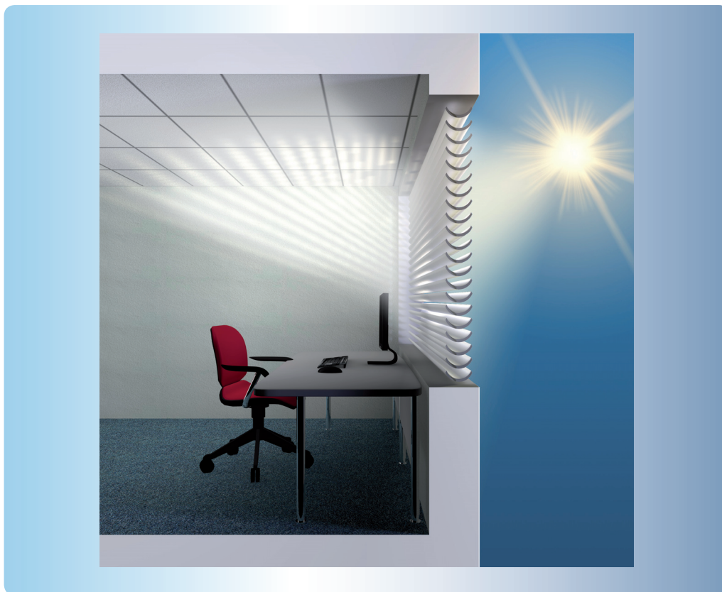
Fig. 35: Optimum daylight utilization through louvre angle tracking
