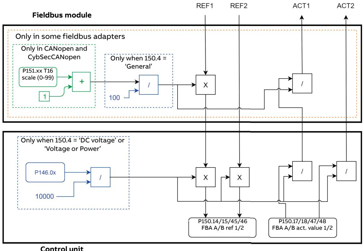
**Example:** PLC reference is 600. Parameter 152.02 FBA A data in1 is set to Ref1 16bit. Reference Ref1/Act1 is scaled first by parameter 151.06 T16 scale since the supply units are identified automatically as Transparent 16 profile. After that the value is scaled in parameter group 146 Monitoring settings, for example using parameter 146.01 Power scaling.
