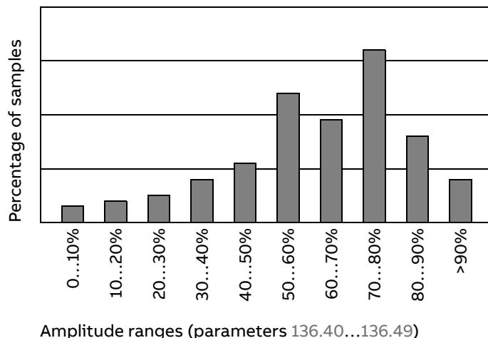
Amplitude logger 1 is fixed to converter current, and cannot be reset. With amplitude logger 1, 100% corresponds to the maximum current of the drive. The measured current is logged continuously. The distribution of samples is shown by parameters 136.20...136.29.
