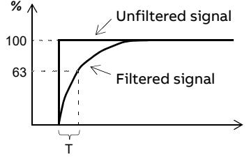
$O = I \times (1 - e^{-t/T})$ <p>I = filter input (step)<br/> O = filter output<br/> t = time<br/> T = filter time constant</p>                                                                  |             |
