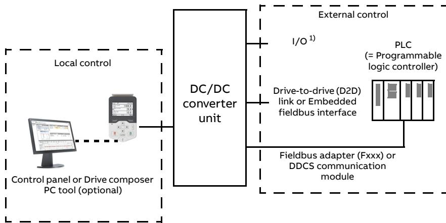
1) Extra inputs/outputs can be added by installing optional I/O extension modules (FIO-xx) in the option slots of the control unit.
