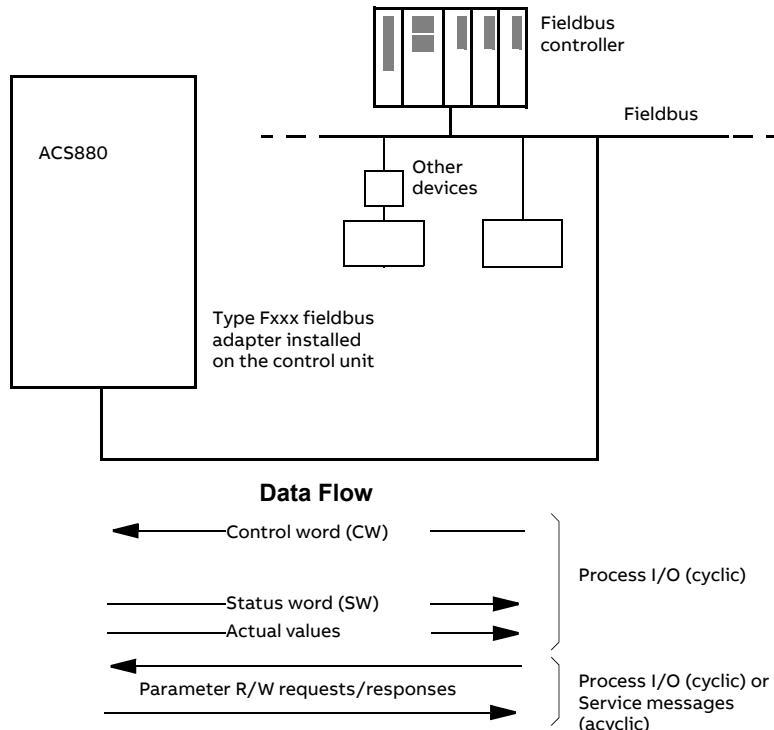
The DC/DC converter unit can be set to receive its control information through the fieldbus interface, or the control can be distributed between the fieldbus interface and other available sources such as digital and analog inputs.
