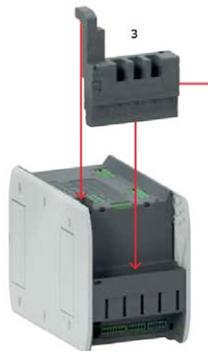
Fig. 5.2 Ekip Signalling and Com -modules are mounted to Bypass isolation automatic transfer switch with a auxiliary power supply module, OXEA1.
