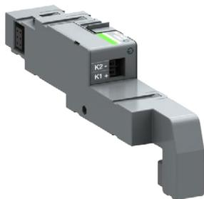
Fig. 5.6 Auxiliary power supply module, type OXE1, is needed when Ekip Signalling, Com and Link -modules are mounted to TruCONTROL\_
