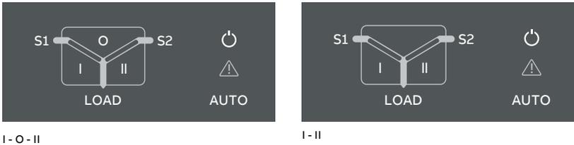
Fig. 3.5 On left: LEDs in ZTBSD/ ZBTSC2 delayed/closed transition, I - O - II. On right: LEDs in ZBTS, open transition I - II.
