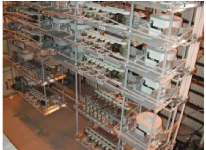
Fig.3 View of six-pulse Back-to-Back bridges, two auxiliary modules and two test modules
