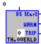
Figure 183: Function block thermal overload protection
