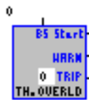
Figure 184: Function block thermal overload protection
