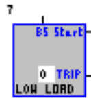
Figure 224: Function block low load supervision
