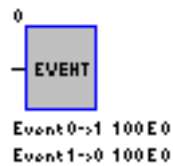
Figure 236: Function block event generator
