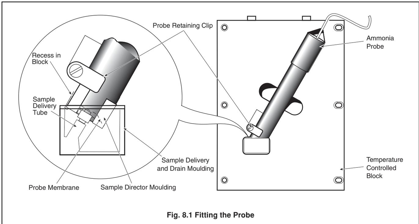
Fig. 8.1 Fitting the Probe
