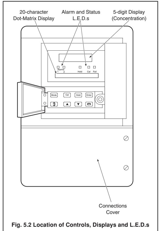
**Fig. 5.2 Location of Controls, Displays and L.E.D.s**
