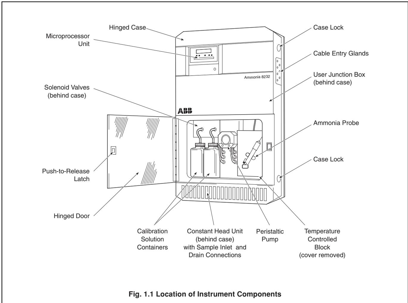
Fig. 1.1 Location of Instrument Components
