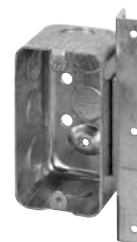
T Type bracket Positions handy box against the face and side of stud. 5\frac{1}{2} " long x \frac{7}{8} " wide
