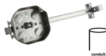
54151 J 1/2 Mounted on 6010-DW bar adjustable 10 1/2" to 18 1/2". Offset for 1/2", 3/4" or 7/8" plaster. Maximum horizontal positioning. 3/8" fixture stud.
