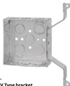
DV Type bracket Mounts box offset from stud 1\frac{1}{2} ". 6\frac{1}{4} " long x 1" wide x 1\frac{1}{2} " offset
