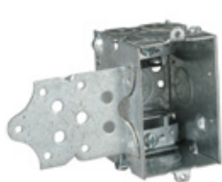
S or B Type bracket Mounts to face of stud. Used on switch, handy or square boxes. 2" long x 2\frac{1}{8} " wide
