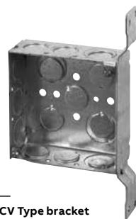
CV Type bracket (outlet boxes) Mounts to flat side of metal studs or wood studs. 7\frac{3}{8} " long x 1" wide x \frac{3}{8} " offset
