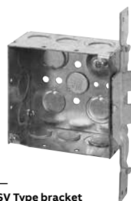
SV Type bracket Mounts box to side of stud with positioning spikes. 7\frac{3}{8} " long x 1" wide x \frac{3}{8} " offset
