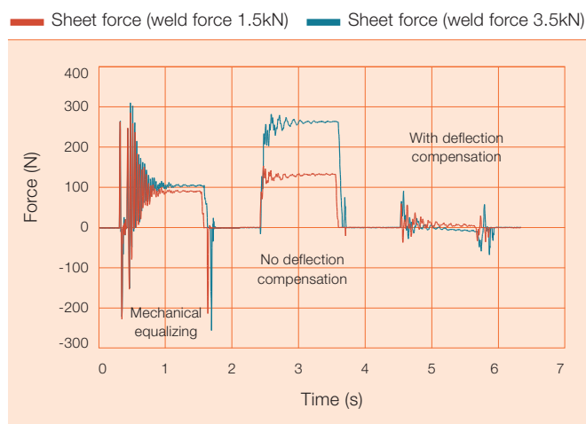
5 Force in metal sheet for welding forces of 1.5 + 3.5 kN
