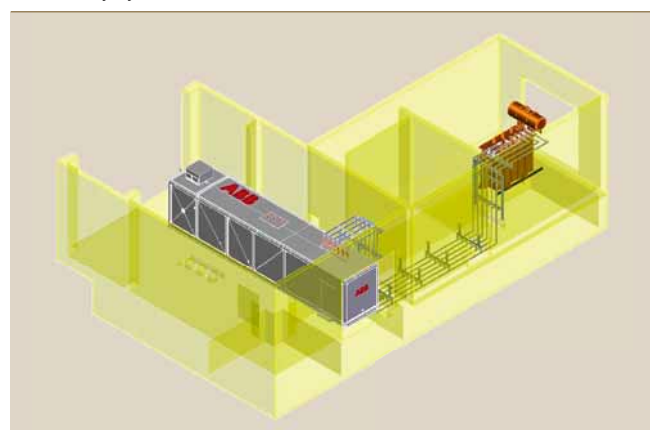
9 3-D model showing the complete installation with an 11.6 MVA transformer, a container comprising converter, cooling unit and auxiliary systems.
