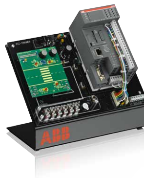
ABB PLC trainer AC500 with plug-on traffic light module
