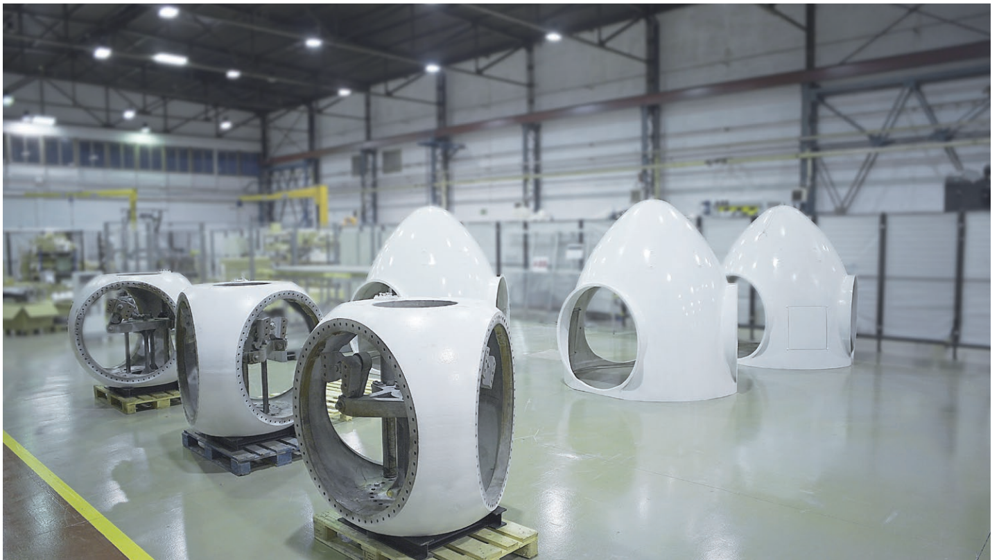
Wind turbine dismantled components to be remounted after the retrofit by ABB's Service Center of Excellence
