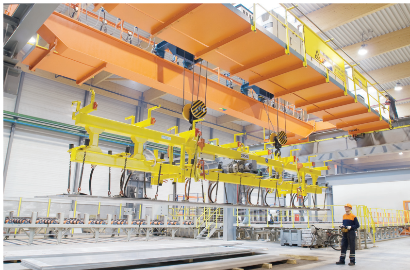
Master-follower arrangement and synchro control provided by ABB industrial drives, such as this one at an aluminium production facility in Belgium, ensure that the crane hooks operate in synchronisation, to avoid any slipping of the load.
