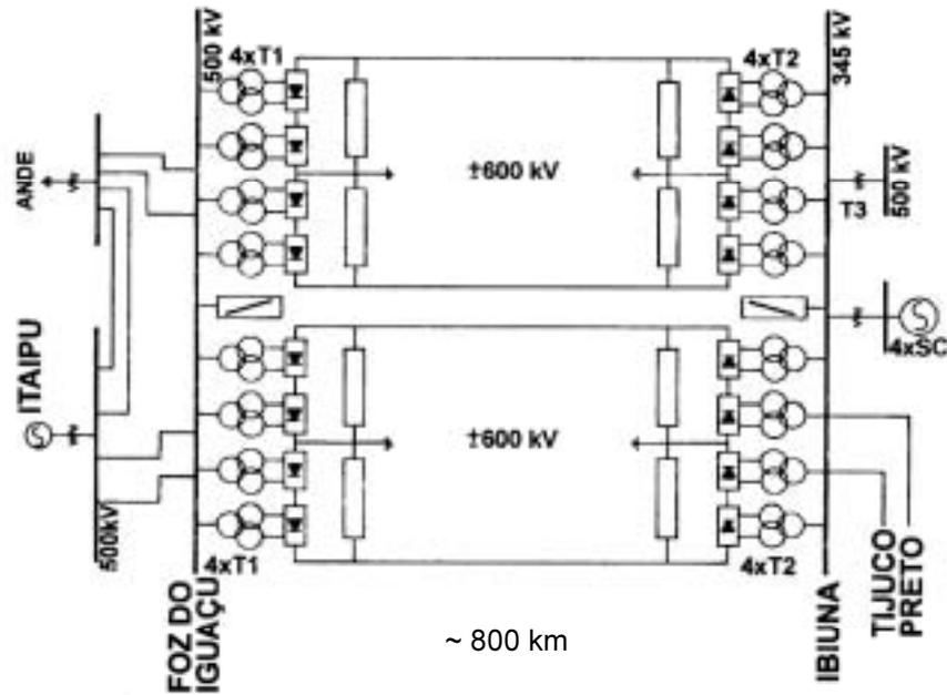
Fig.3 The Itaipu HVDC Transmission
