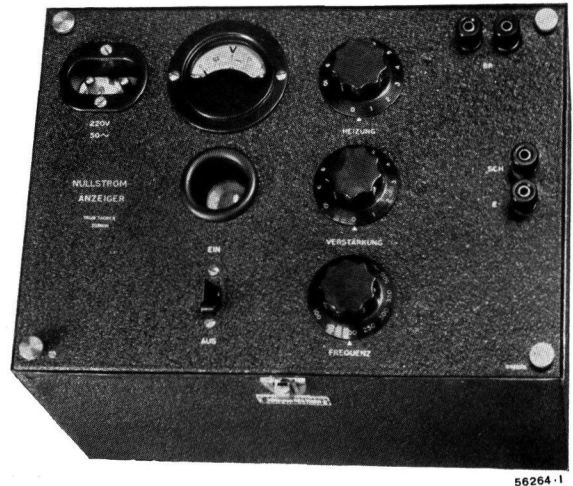
Fig. 3. — Zero instruments by Messrs. Trüb, Täuber & Co. A. G., Zürich, for a.-c. currents and frequencies of 100 to 500 cycles.
