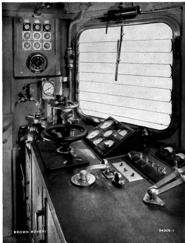
Fig. 9. — Driver's cab for one-man control of the locomotive.
