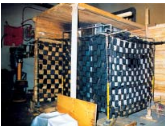
Internal arc test indicators arrangement.
