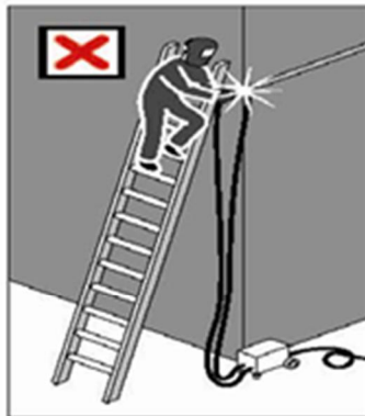
Performing hot work from ladder
