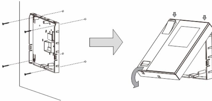
1. Affix the bottom of the device to the wall.
