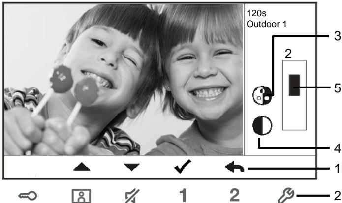
Fig. 3 Display and volume setting during a call
