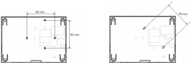
1. The bottom of the device has screw holes for fastening on the wall according to the illustrations above.
