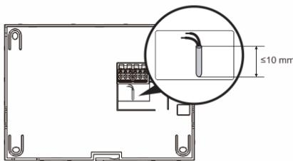
Affix the bottom of the device and connect it according to the illustration. The insulated section of the cable end must not be longer than 10 mm.
