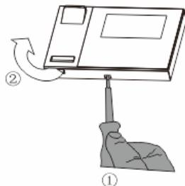
Open the housing of the panel by pulling the clamp at the bottom of the device.
