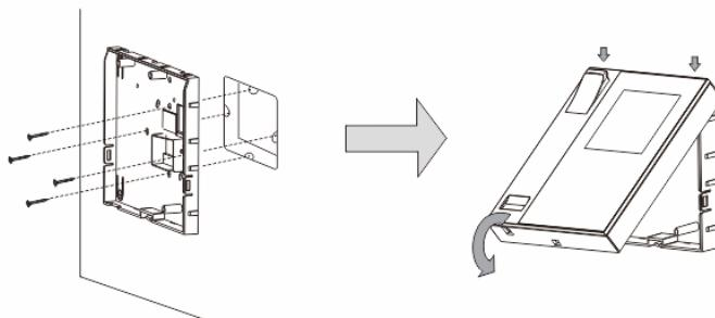
1. Affix the bottom of the device to the existing flush-mounted box.
