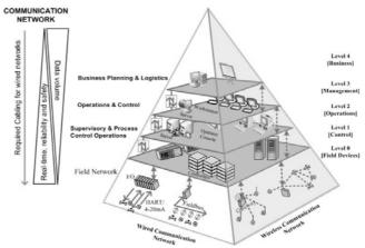
Fig. 1. Automation pyramid based on ISA-95 functional hierarchy.
