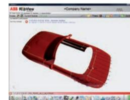
With RobView 5 you can manage your paint installation, whether it is one or many robots, visualize the complete paint process, and operate and supervise your paint robot cell. A basic version of RobView 5 is bundled with all IRC5P paint robots, free of charge\*. It is an affordable graphical user interface for low budget installations. However, it is scalable and expandable with plug-in options for large and advanced installations.
