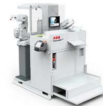
It replaces manual tending and other feeders when a short cycle time is required. FlexLoader FP 300 is quickly and easily installed or moved. The whole cell, including the robot, is built on a single baseplate and takes up very little space.
