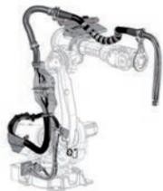
External DressPack with a retract arm pulling the cables away from the wrist. Minor individual adjustment needed for DressPack.
