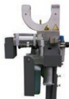
The robot control system operates and supervises the cleaning operation to ensure it does not start until the torch is clamped in the correct position. This guarantees that no vibrations or shocks reach the robot and the torch is locked in the same position every time for more precise cleaning and less wear on the parts being cleaned.
