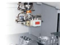
RobotWare Force Control will greatly facilitate the use of robots for tasks that needs "touch sensing", like assembly, fixturing, product testing etc. The option is based on the force control concept, i.e. a robot control strategy where the robot movements are adapted to the feedback from a force sensor. Thus the robot can automatically search for the correct location, and assemble parts using intelligent force/torque motion without the risk for jamming or part damage.
