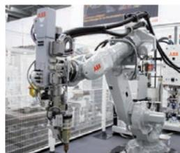
RobotWare-Dispense can be used for different types of dispensing processes. It is a software option typically used for gluing, sealing, spraying and other similar processes, but can also be useful in a wide spectrum of other applications.
