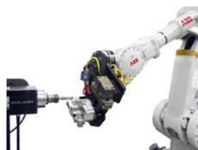
Enables easy teaching and automatic path generation of complex part surfaces and edges for machining processes like polishing, deburring, grinding. Forces are also controlled during the processing instead of the conventional position control of the robot which makes it more sensitive and increases the quality of the finished parts. Suitable function packages are available for various machining robots of ABB.
