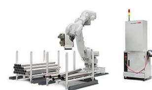
It handles workpieces that are in disarray just as well as those arranged in layers, with or without dividers.
