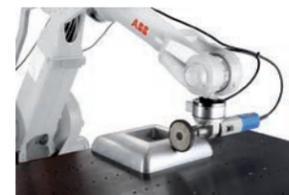
Conventional robotic solutions are controlled by predefined paths and speeds. However, with Integrated Force Control, the robot reacts to its surrounding and can deviate from its programmed path or speed based on feedback from the force sensor. It is possible to automate complex tasks which previously required skilled personnel and advanced fixed automation.
