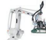
PalletPack is a package of pre-engineered products to make end-of-line and bag palletizing solutions more accessible and easier to use. The package includes robot, gripper and easy-to-use wizard on Flexpendant for setting up different palletizing tasks. A PLC including safety is included for control of the complete line.
