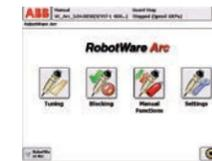
RobotWare Arc comprises a large number of dedicated arc welding functions. It is a simple yet powerful program since both the positioning of the robot and the process control and monitoring are handled in one instruction.
