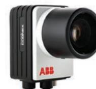
Compact smart cameras that are easily programmed in RobotStudio® together with the robots makes vision guided robots viable for any user. The vision system is highly robust and proven in industrial solutions under tough conditions. The product comes complete with cables, filters, lenses, cameras and software.
