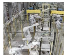
Conveyor Tracking (also called line tracking) is the function which makes the robot follow a work object on a moving conveyor. While tracking the conveyor, the programmed TCP speed, relative to the work object, will be maintained even when the conveyor speed is changing slowly.
