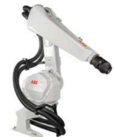
Bending backwards possibility on axis 3 (may be limited by the hose guiding on the robot)
