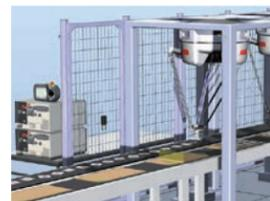
Picking PowerPac is an offline tool that simulates PickMaster 3 in picking applications. The PowerPac offers ease of use configuration of a picking application which can be simulated and fully optimized before being downloaded into PickMaster 3 for real production.
