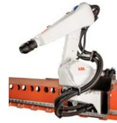
Bending backwards possibility on axis 3 (may be limited by the hose guiding on the robot)
