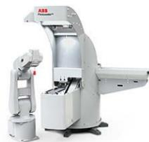
It's compact but has a wide range of functions. Even if you're only processing two workpieces, FlexLoader FP 100 is a good investment. It completely replaces conventional bowl feeders. The buffer is located outside of the cell, making it simple to tip in workpieces.
