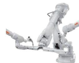
A MultiMove system is a system where a common controller controls up to four robots, each equipped with its own drive module. MultiMove system exists in two different modes – Independent and Coordinated. With MultiMove Independent, the robots run independently of each other, i.e. controlled by separate RAPID tasks. It is also possible to run positioners independently (controlled by separate RAPID tasks).
