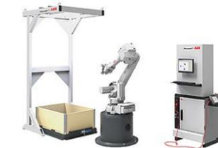
It is a fully automated feeder for all kinds of workpieces, picking straight from the pallet as long as the workpieces are semi-oriented or arranged in layers, with or without dividers.
