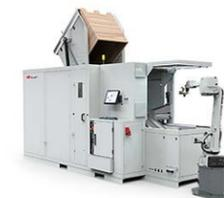
The cell will with high speed and great accuracy handle workpieces up to 250 mm long and approximately 3 kg in weight. Workpieces are either tipped directly onto a buffer conveyor, or a pallet tipper can be connected.
