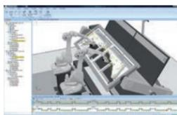
ArcWelding PowerPac is an add-in to RobotStudio that makes it fast and easy to program arc-welding applications. It includes VirtualArc, an expert system that makes it possible to determine the process parameters necessary to achieve a particular welding result. Use of ArcWelding PowerPac makes it easy to make sure that the optimum tool angles are always used, resulting in higher quality welds and shorter cycle-times.
