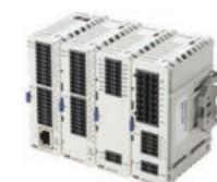
ABB Robotics has expanded the I/O communication capabilities of IRC5 and the I/O system are based on a compact modular design with big improvement in flexibility, easiness and reliability. The system consist of a base unit serving as the minimum configuration. It is equipped with industrial network connectivity, 16 digital inputs, and 16 digital outputs.
