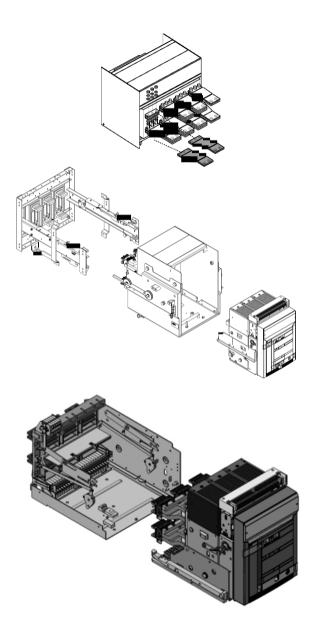
Hard Bus Retrofill (HBR): The obsolete circuit-breaker is totally removed and substituted with the Emax circuit-breaker. The kit contains custom designed and preconfigured busbars and covers to adapt the new circuit-breaker to the existing busbars.
