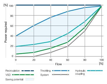
Power consumption for various pump control methods
