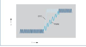
Typical torque (T) response of a DTC drive, compared with flux vector control with open loop pulse width modulation (PWM)
