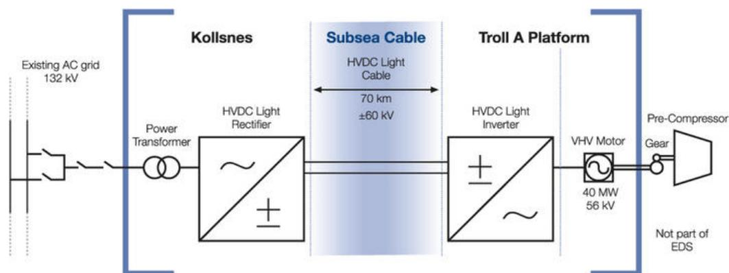
Figure 3 Troll A application single line diagram.
