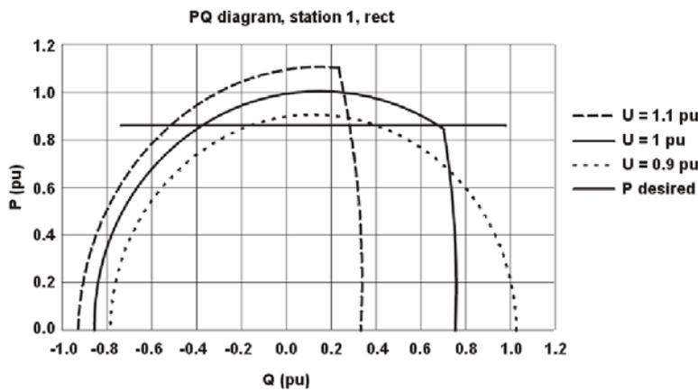
Figure 2 Typical P/Q diagram
