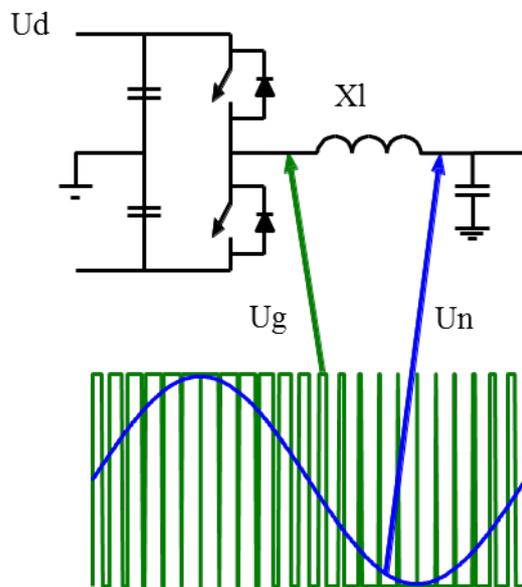
Figure 1 shows one phase of a VSC converter using PWM
