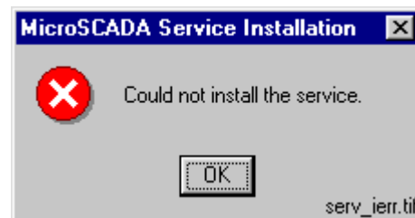
Fig. 7.5.-1 The MicroSCADA service installation has failed
