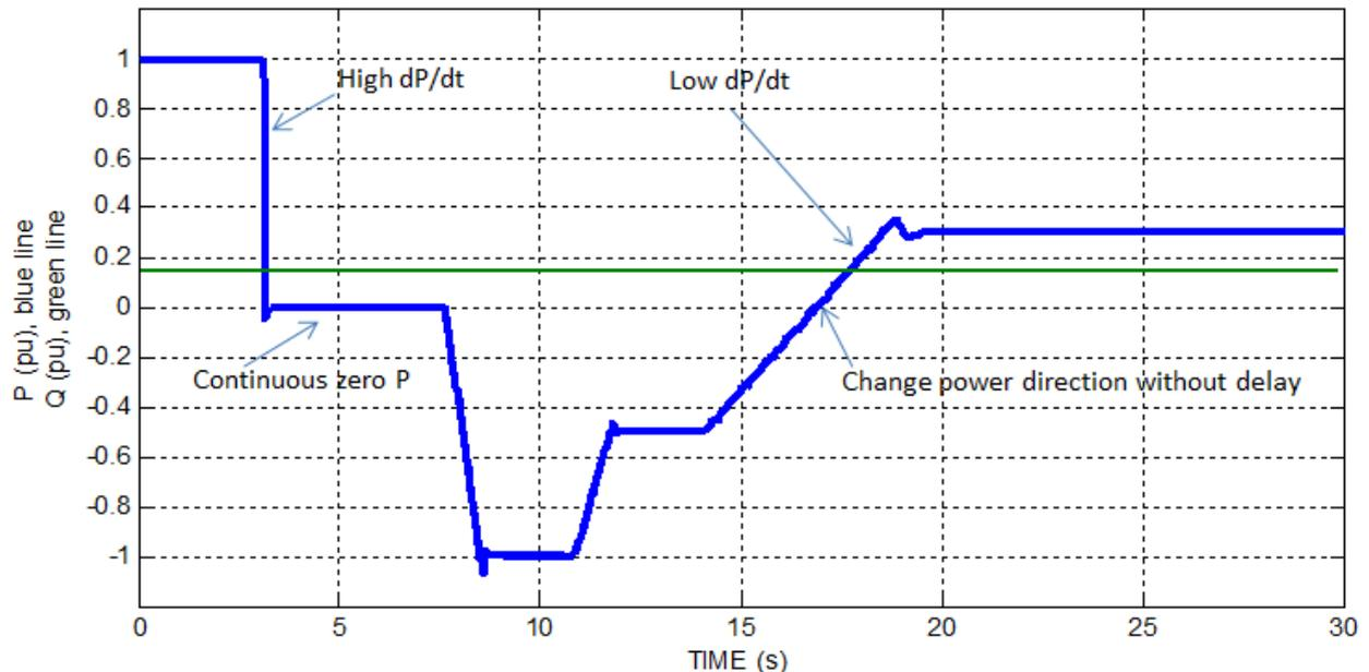
Fig. 1. Example of operating active and reactive power
