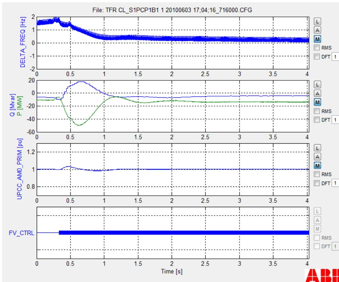
Fig. 4. Performance of VSC HVDC in providing primary and secondary control – control over frequency
