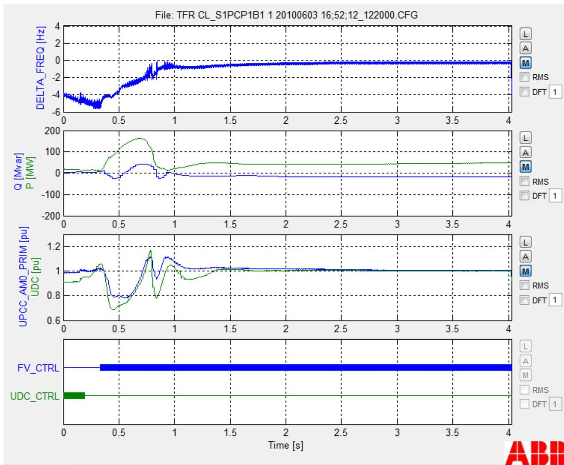
Fig. 3. Performance of VSC HVDC in providing primary and secondary control – control under frequency
