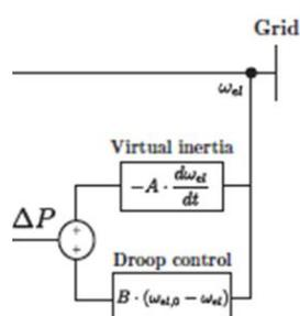
Fig. 2. VSC Converter Supporting Frequency Control by power dispatch mode
