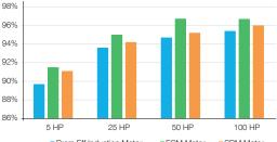
Prem Eff Induction Motor FCM Motor SRM Motor Figure 10: A Comparison of the Efficiencies of All Three Motors
