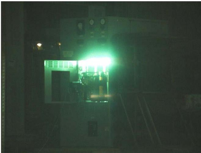
Fig. 18. Line side fault with HSGS protection
