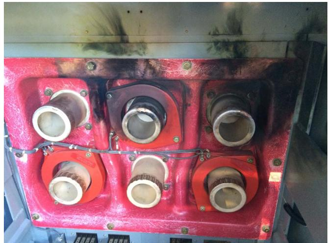
Fig. 19. Damage to Main Compartment after Test 7
