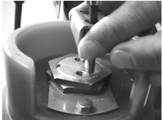
Figure 5.3 Removing connection bars.
