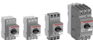
Manual motor starters are electromechanical protection devices for the main circuit. They are mainly used to switch motors ON/OFF manually and to provide fuseless protection against short-circuit, overload and phase failures. Fuseless protection saves costs, space and ensures a quick reaction under short-circuit condition by switching the motor off within milliseconds. Starter combinations are setup together with contactors and are available with screw or push-in spring terminals.
