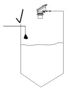
THIS IS CORRECT AS THE FILLING POINT IS NOT OBSCURING THE KSONIK MICRO'S LINE OF SIGHT 4. If the KSONIK MICRO LP is in a coned vessel, it must be positioned over the cone. This ensures that the Transducer receives the true echo and not one from the sides of the cone.
