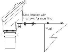
3. The KSONIK MICRO LP must be perpendicular to the material it is measuring with a clear line of sight and must not be above beams or filling points.
