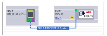
IO addressing is assigned automatically to FSPS. This can be seen in Device view (highlighted red box).
