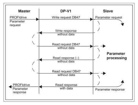
The messaging employs DP-V1 data units. The PROFIdrive parameter request is included within the DP-V1 request as data. Likewise, the DP-V1 response contains the PROFIdrive parameter response as data.
