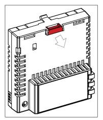
2. Install the module carefully to an option module slot of the drive. See the drive hardware manual.
