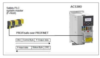
The FSPS-21 module is installed on the ACS580 drive. The safety PLC is connected to the FSPS-21 module. The safety PLC activates safety functions via the PROFIsafe communication bus.
