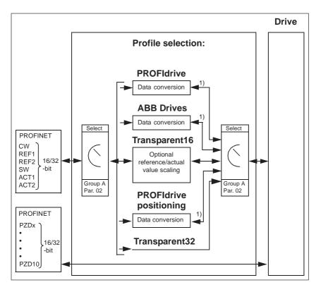
**Note:** The diagram is applicable only when PPO messaging is used. If Standard Telegrams (ST) are used, the communication profile is selected automatically.
