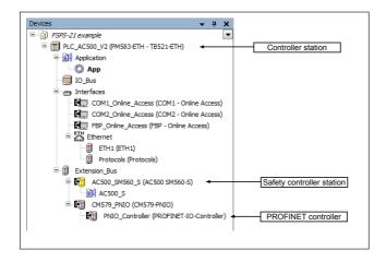
**Note:** Make sure that the "Enable debug" setting is On for the safety controller station, if you want to view or debug the PLC program after the download.
