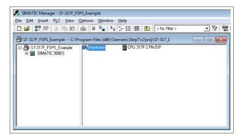
Select the controller station and rail from the catalog and drag them to the project. This example project uses a CPU 317F-2 controller station (V3.2) that is installed in a RACK-300 Rail.
