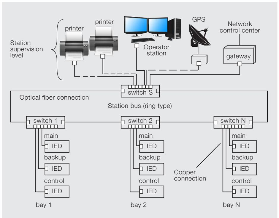
Example of non-redundant station bus
