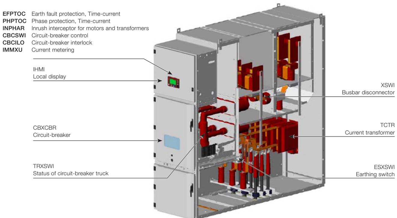
The data model for a medium voltage switchgear unit
