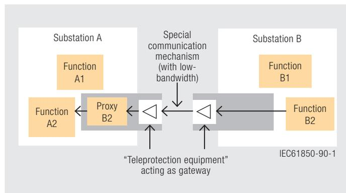
Communication principles based on Standard IEC 61850, between substations
