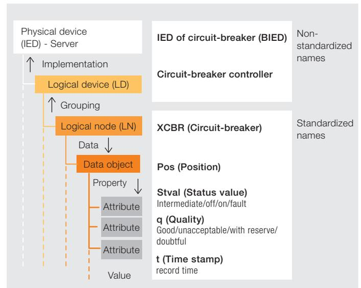
The IEC 61850 object-oriented data model of a physical device
