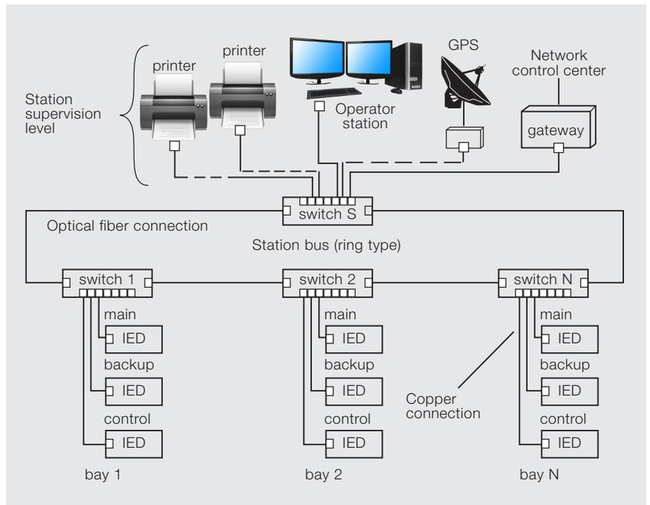
Example of non-redundant station bus
