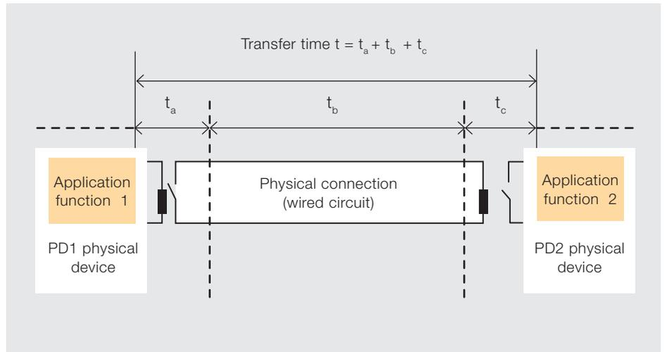
Definition of transfer time with wired circuit (input/output relay)
