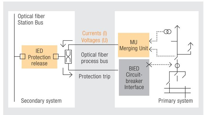
Process bus with "merging" unit (MU), circuit-breaker interface (BIED) and external Ethernet switch
