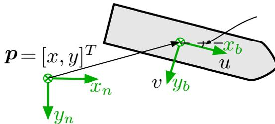
Figure 1: Definition of coordinate systems and velocities
