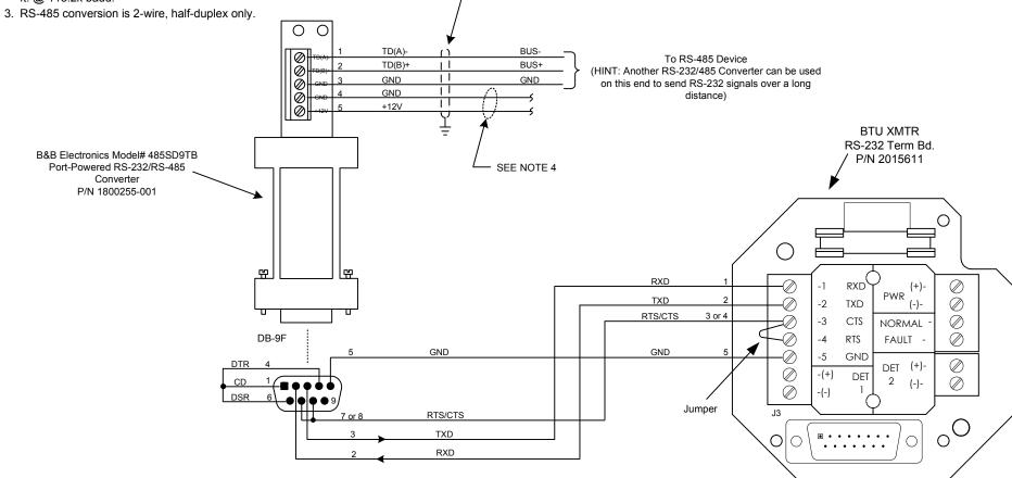
4. No external power is required if two RS-232 output Handshake lines are available. External +12VDC can be applied to the pins on the RS-485 side between terminals +12VDC and GND, when handshake lines are not used.
