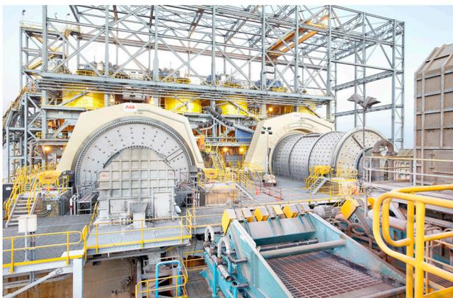
Figure 5. Two gearless mill drives at Esperanza copper mine in Chile.
