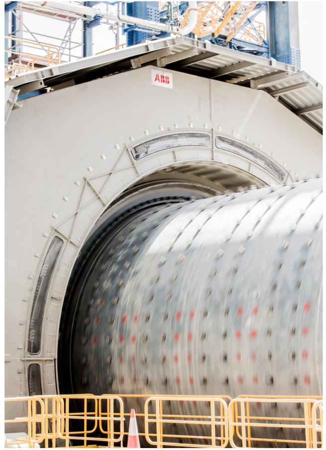
Figure 3. Gearless mill drive (GMD) in Sierra Gorda, Chile.
