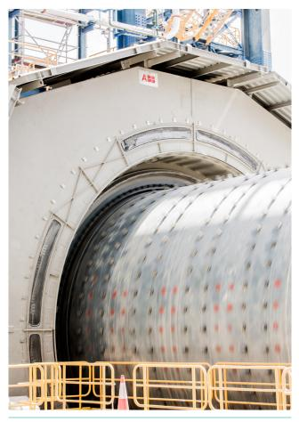
Figure 3. Gearless mill drive (GMD) in Sierra Gorda, Chile.
