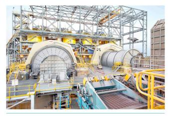
Figure 5. Two gearless mill drives at Esperanza copper mine in Chile.
