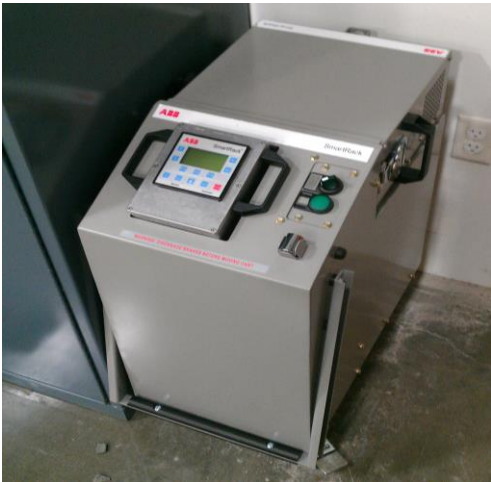
Figure 9: Properly Stored SmartRack™
