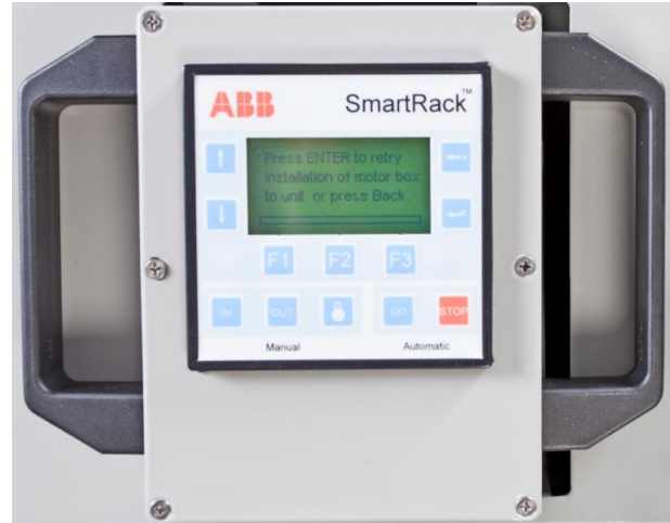
Figure 7: Control Box Handles
