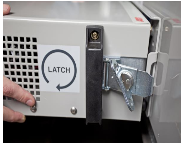
Figure 19b: Installation of Motor Box 2
