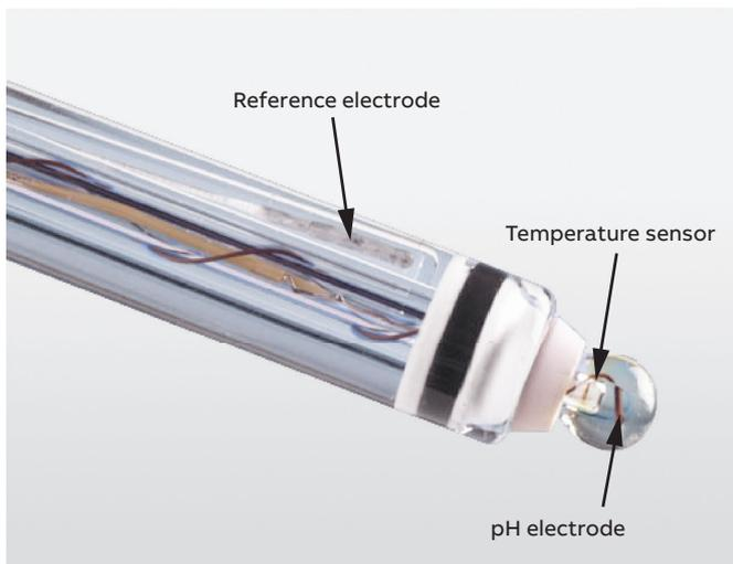
Balanced position of sensing elements
