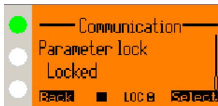
LCD panel with locked parameters
