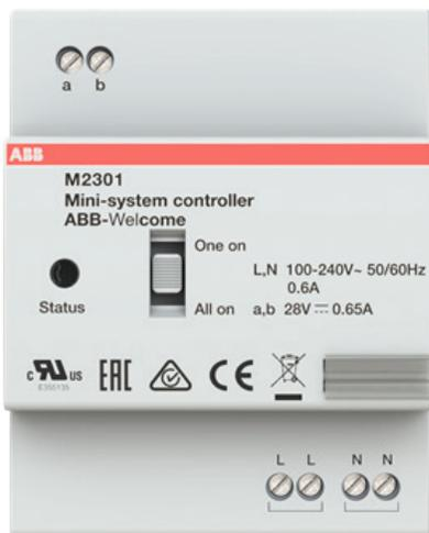
Serves as the brains and primary source of power of the door entry systems and manages communication between all components – outdoor stations, indoor stations, guard units, and other system components. It can also serve as auxiliary BUS power supply.
