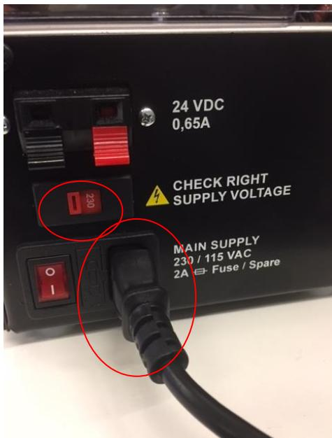
Check that the Input voltage switch (115V/230V) is set according to the supply voltage. For more information check “AC input (supply) connection” in the Technical data section. Switch on the demo using the mains switch.
