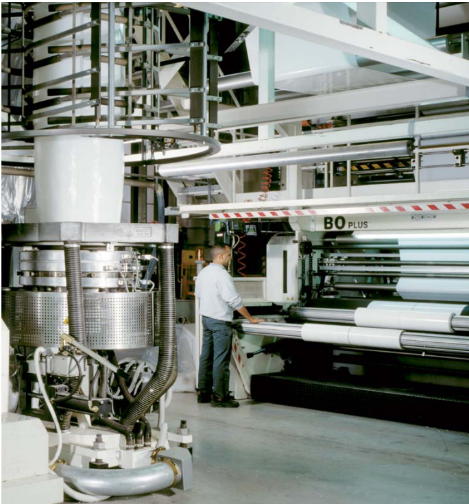
Winding of the flatten blown film.
