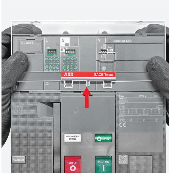
**7** Lift the springs charging lever and by means of the cross screwdriver unscrew the screw located below the springs charging lever fixing the circuit breaker cover to the circuit breaker main structure.
