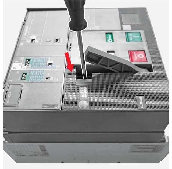
**8** By means of the cross screwdriver unscrew the 2 screws located in the lower part of the circuit breaker fixing the circuit breaker front cover to the circuit breaker main structure.
