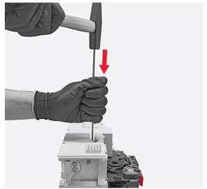
Put the circuit breaker with front up and push the rod as indicated by the arrow until the pin comes out from the hole left by the cover cap on the right side of the circuit breaker and after remove the rod.
