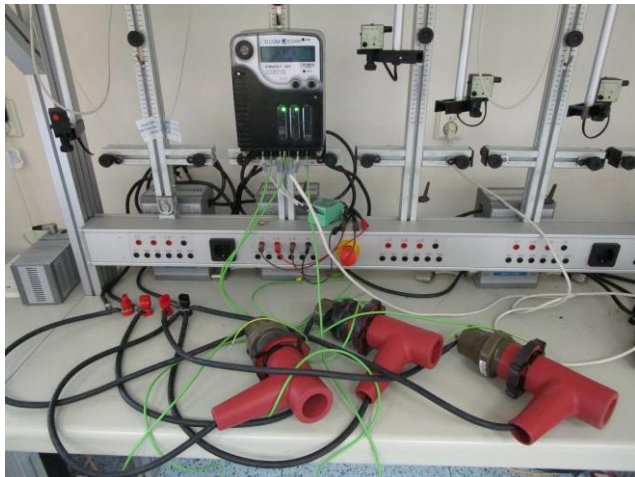
Fig. 2 Revenue energy meter connected to LPCTs during the accuracy test
